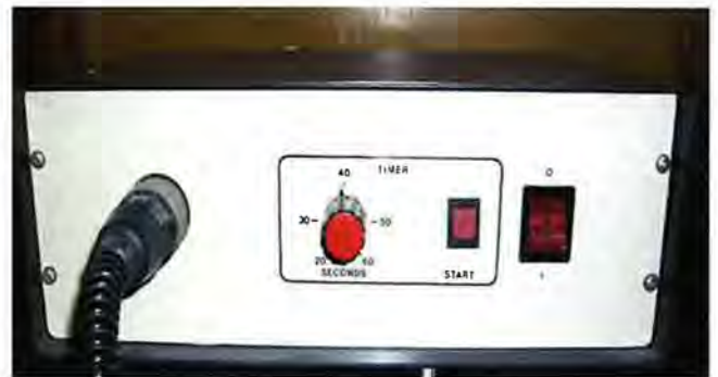
Fig. 5 Details of the prototype light curing (activation) unit used in the placement of the 'first in man' visible light cured composite.
